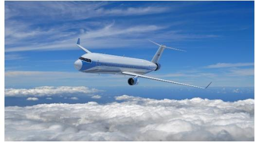
Concept of Single-aisle Turboelectric Aircraft with Aft Boundary Layer propulsion (STARC-ABL)
