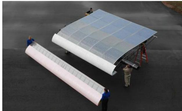
Aurora engineers display a test section of a wing designed for a large solar-powered aircraft. The section, built entirely of advanced composite materials and covered with solar cells, represents about 5% of the span of the actual aircraft. It is shown for comparison with the center wing section of the world record holding Daedalus human-powered aircraft.
