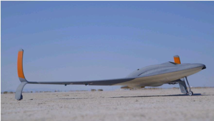
To realize the joint goal to design and develop an advanced 3D printed demonstration aircraft, the final UAV - which has a 3m (9ft.) wingspan and weighs only 15kg (33lb.) - leveraged 3D printing for 80 percent of its design and manufacture and is built on the expertise of Aurora Flight Sciences' aerospace and Stratasys' additive manufacturing.
