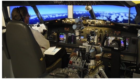
An IT specialist at the John A. Volpe National Transportation Systems Center flies a Boeing 737-800NG simulator with Aurora's ALIAS technology demonstration system as his co-pilot.
