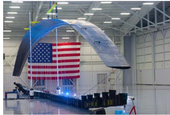
Aurora performed a limit load test of the Orion wing at its Columbus, Mississippi location.
